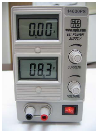
Figure 5: Correct output from power supply before connecting to IMU.
