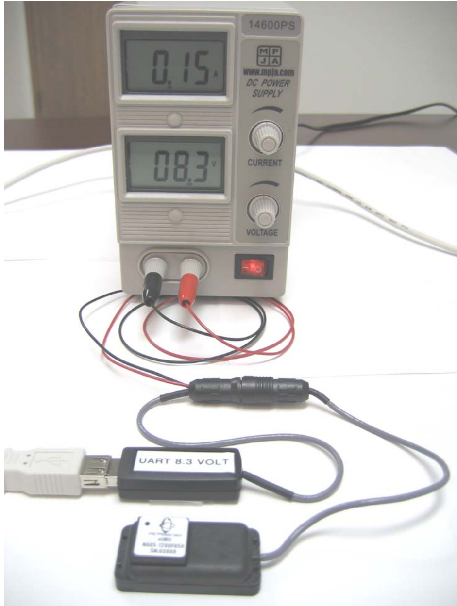
Figure 6: Power supply, IMU and USB interface board connectivity.
